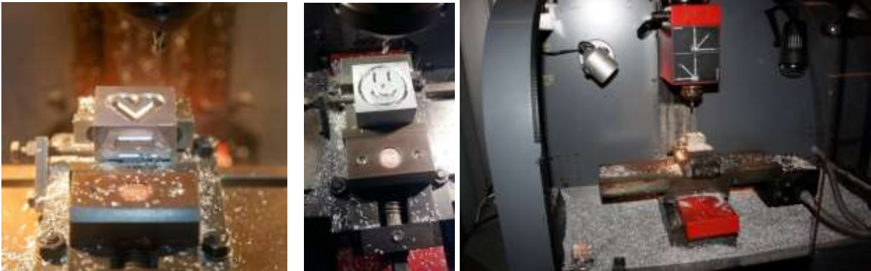
Creating a part on an EMCO computer numerical control (CNC) cutter workbench in Tehnobuss
